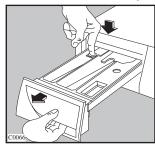
To aid cleaning, the top part of the additive compartment should be removed. Clean all parts with water.
